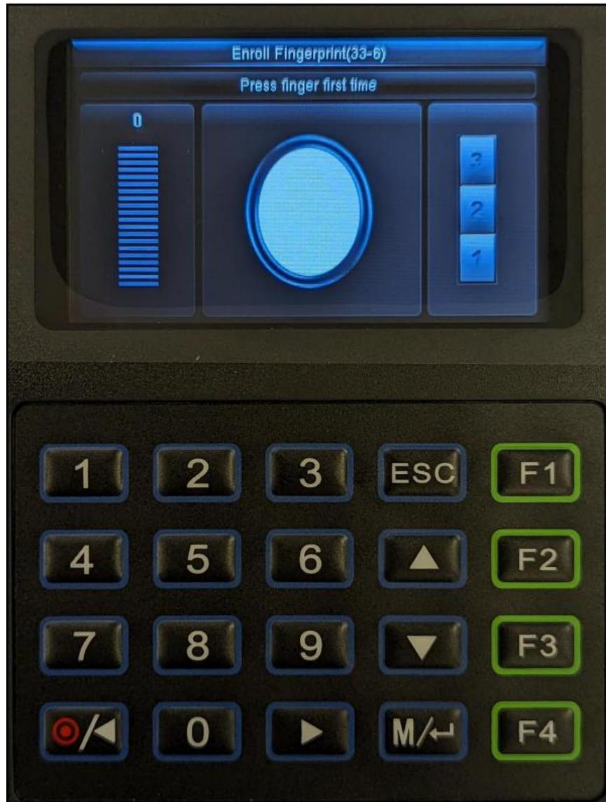
11. **Test Punch** – Have the employee record a punch via fingerprint to confirm whether the print will be accepted by the scanner.
