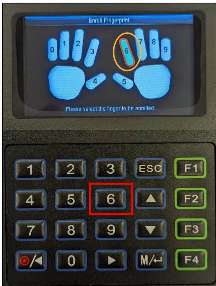
10. **Scan Finger** – Following the directions provided on the screen, scan the finger three times until it is successfully enrolled.
